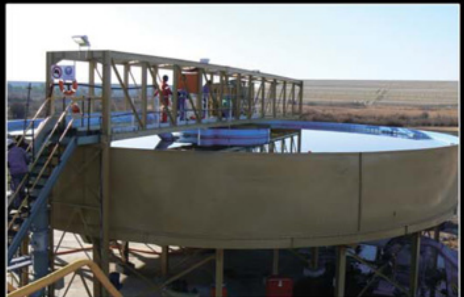
21m \phi thickener from bolted construction
