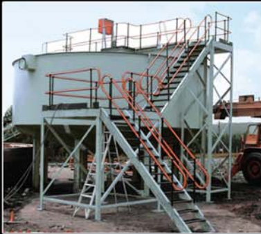
8m Thickeners in operation
