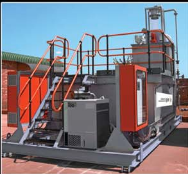
Skid mounted Flocculant Plant
