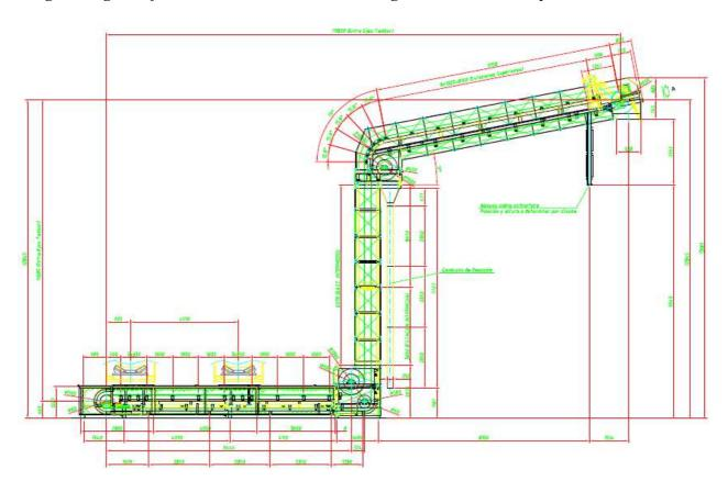
Longer loading area for 6 inlets, short inclined part and short outlet area
