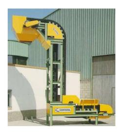
After the horizontal loading section a deflection disc bends the belt into the vertical path of lift. The upward and downwards strands are encased from the bottom to the top. Substructures or support rollers will depend on each project.
