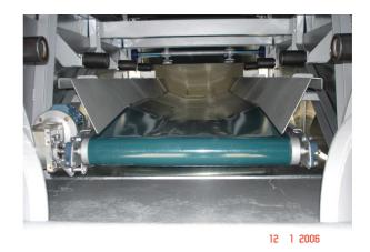
Lateral deflection discs turn the belt from the horizontal back to the vertical.
