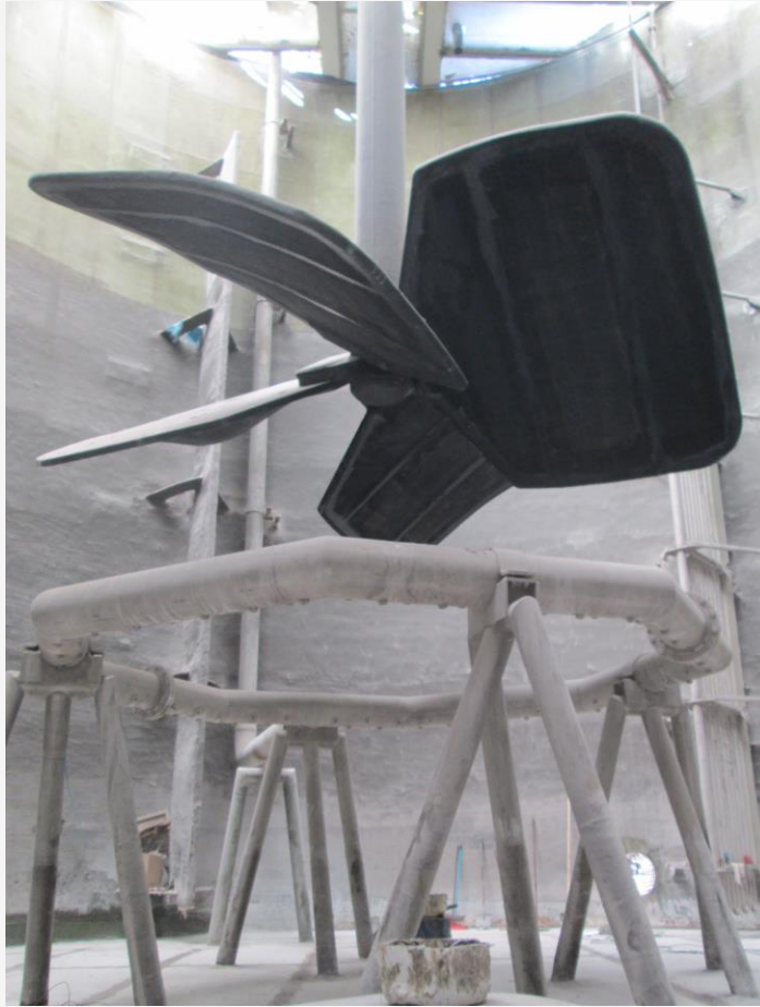
Bioleaching Copper Reactor 110kw, 5.8m dia
