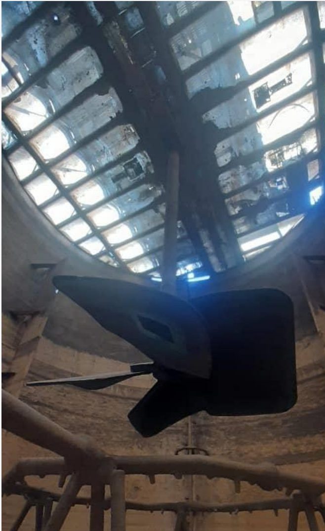
▲ Bioleaching Copper Reactor 110kw, 5.8m dia
